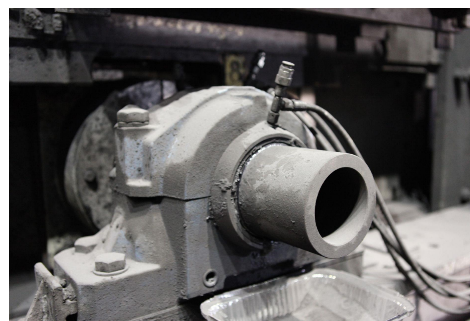
A lubrication point on one of the Grate support shafts.
