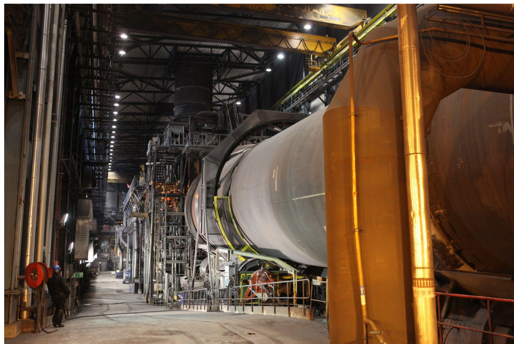
The LKAB KK4 travelling grate (background) and rotary kiln (foreground), which together form the warm process of the pelletizing plant.
